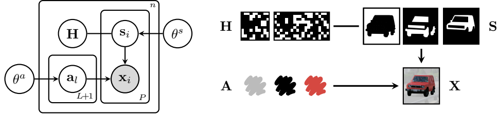
Figure 4: A model of shape and appearance. Left: The joint model. Pixels \mathbf{x}_i are modeled via appearance variables \mathbf{a}_l . The model’s belief about each layer’s shape is captured by shape variables \mathbf{H} . Segmentation variables s_i assign each pixel to a layer. Right: Schematic for an image \mathbf{X} .
