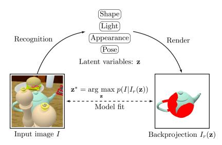
Fig. 1: Illustration of our inverse-graphics solution. Given an image, the recognition models of shape, lighting, appearance and pose initialize the latent variables. Then, the differentiable renderer generates an image which is fitted by optimizing over the latent variables  $\mathbf{z}$  that best match the input image, i.e.  $\mathbf{z}^* = \arg \max p(I_{GT}|I_r(\mathbf{z}))$ . Detected occlusion mask is illustrated with red
